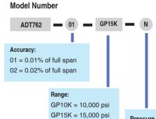
Pressure port type: N - 1/4 NPT female N2 - 1/2 NPT female B - 1/4 BSP female
